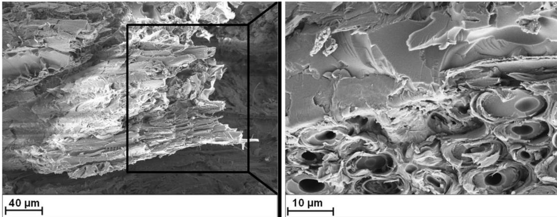
**Figure 2.** Scanning electron micrographs showing the fracture surfaces of 60wt% SWF-filled composites prepared at a temperature of 170°C and under a pressure of 80bar.
