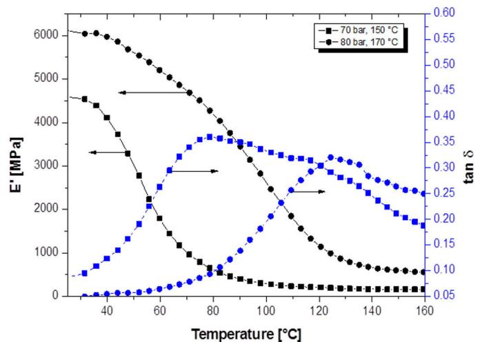
**Figure 4.** Effect of processing on the thermomechanical properties of the SWF/Acrodur composites with 60wt% of SWFs.  $E'$ : Storage modulus.  $\tan \delta$ : Damping factor.
