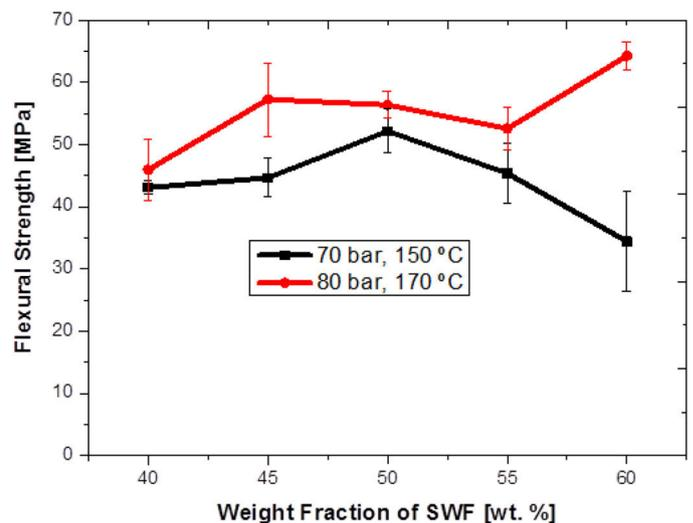
**Figure 1.** Flexural strength values of short wood fiber/Acrodur composites with different fiber content and after undergoing treatment (either at 70bar and 150°C, or at 80bar and 170°C). SWF: Short wood fiber.
