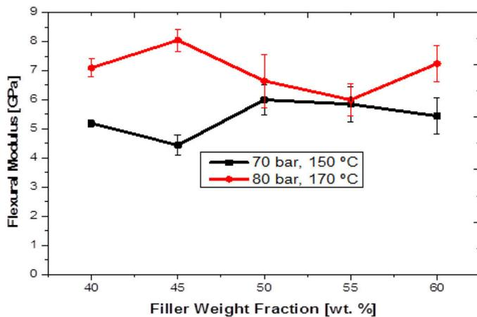
**Figure 3.** Flexural modulus values of the SWF/Acrodur composites.
