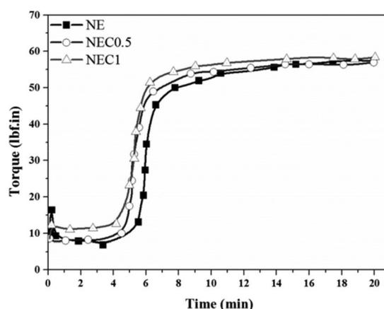
**Figure 1.** Cure curves for elastomer-blend nanocomposites with different carbon nanotube (CNT) loadings. NE: Natural rubber/ethylene propylene diene monomer (NR/EPDM). NEC0.5: NR/EPDM with 0.5wt% CNTs. NEC1: NR/EPDM with 1wt% CNTs. lbf.in: Pound-force inch.
