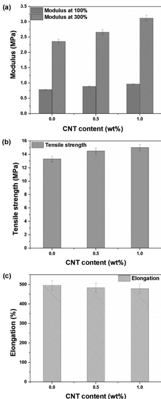
**Figure 2.** The effect of CNT loading on the mechanical properties of NR/EPDM/CNT nanocomposites. (a) The modulus at elongation values of 100 and 300%, (b) tensile strength, and (c) elongation at break for nanocomposites with CNT loadings of 0, 0.5, and 1wt%.
