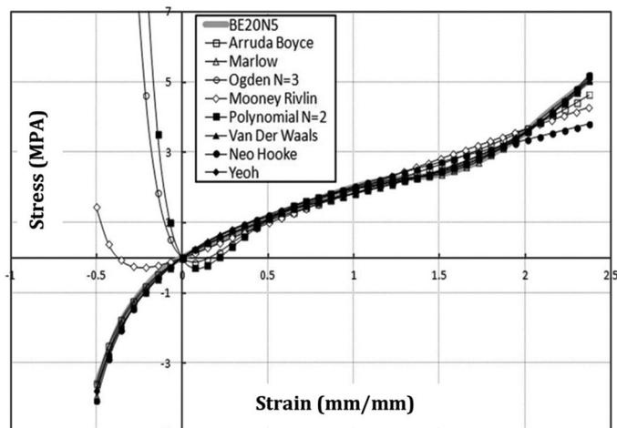
**Figure 3.** Experimental stress-strain data fitted to hyper-elastic models for the BE20N5 nanocomposite.<sup>10</sup>
