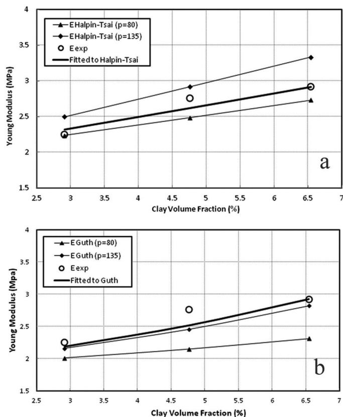
**Figure 2.** Comparing experimental Young’s modulus values for BE20N5 with the values estimated through (a) the Halpin-Tsai relation and (b) the Guth model.<sup>10</sup> p: Aspect ratio.
