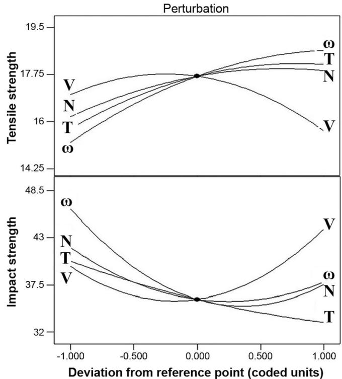
**Figure 3.** Effect of FSP parameters on the mechanical properties of the nanocomposites: (top) tensile strength; and (bottom) impact strength. Results are shown for the effect of (top) V, N, T, and  $\omega$  on tensile strength and (bottom)  $\omega$ , N, T, and V on impact strength.
