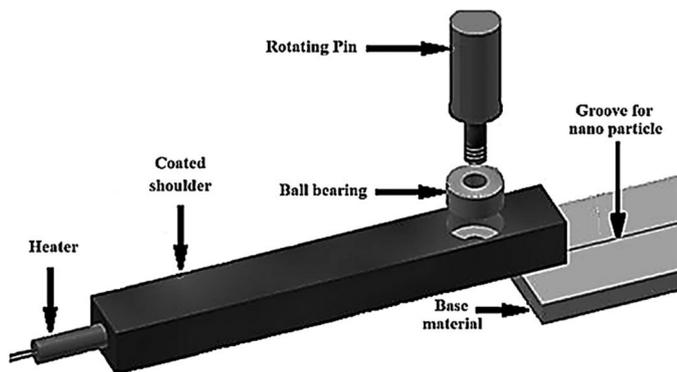
**Figure 2.** Schematic illustration of the new FSP tool used in this study. The tool consists of a pin, Teflon-coated shoulder, ball bearing, and heating system.
