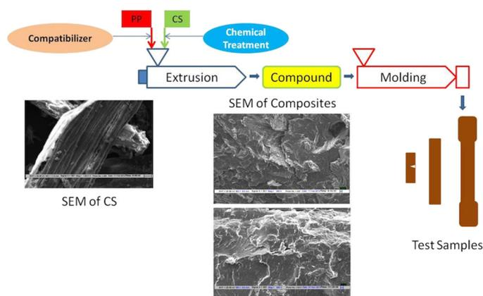
**Figure 1.** Illustration of the full process chain for the preparation of polypropylene/cotton stalk (PP/CS) biocomposites used in this study. Scanning electron microscope (SEM) images of CS and the resultant composites are also shown.
