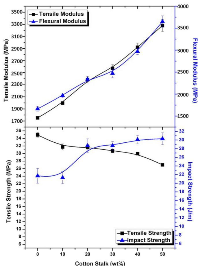
**Figure 2.** Experimentally measured tensile and flexural modulus (top), and tensile and impact strength (bottom) of the PP/CS biocomposites (for CS concentrations up to 50wt%).
