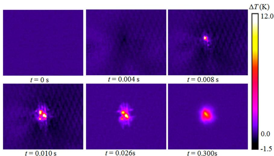
**Figure 2.** Images obtained at six time intervals (0, 0.004, 0.008, 0.010, 0.026, and 0.3s) show a CFRP specimen before, during, and after impact (with an energy of 2.8J). The images, obtained using IR thermography, show the effect that the impact has on the specimen's surface temperature.  $\Delta T$ : Temperature difference in Kelvin, with  $t=0$  used as ambient reference.
