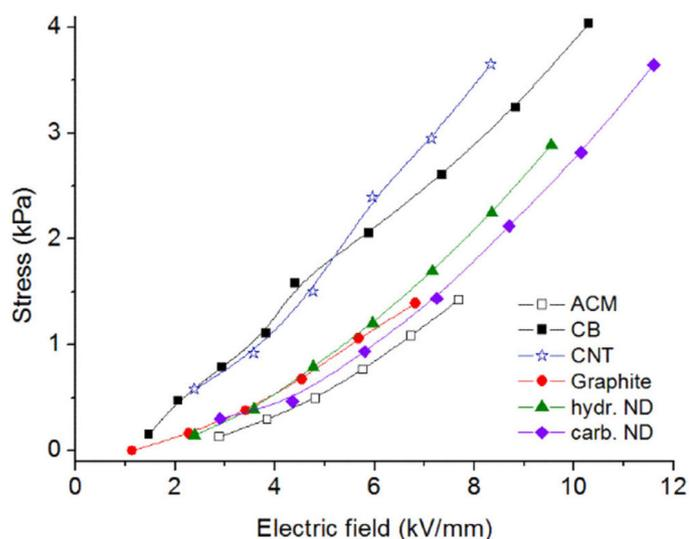
**Figure 2.** Actuation performance of alkyl acrylate copolymer (ACM) containing different carbon-based fillers (at 1 part per hundred rubber). CB: Carbon black. CNT: Carbon nanotube. hydr. ND: Surface-hydrogenated nanodiamonds. carb. ND: Surface-carboxylated NDs.
