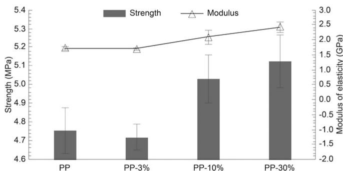
**Figure 2.** Measured flexural properties (strength and modulus of elasticity) of the PP and CNF/PP composites.
