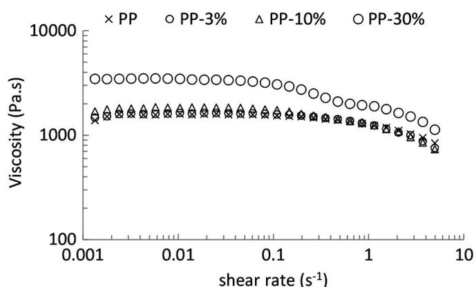
**Figure 1.** Experimentally measured viscosity, as a function of shear rate, of neat polypropylene (PP) and PP composites filled with spray-dried cellulose nanofibrils (CNFs) at loadings of 3, 10, and 30wt%.
