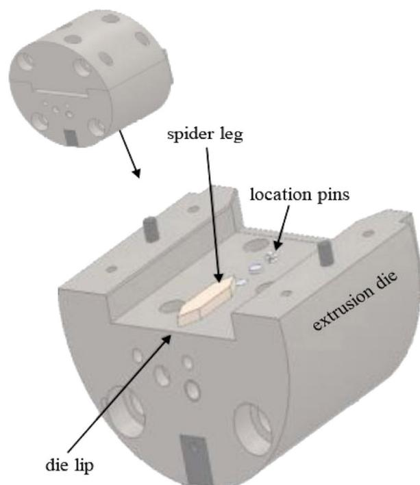
**Figure 1.** Schematic diagram of the extrusion die prototype used in the experimental work. For scale: the spider leg has a length of 28mm (see Figure 2).
