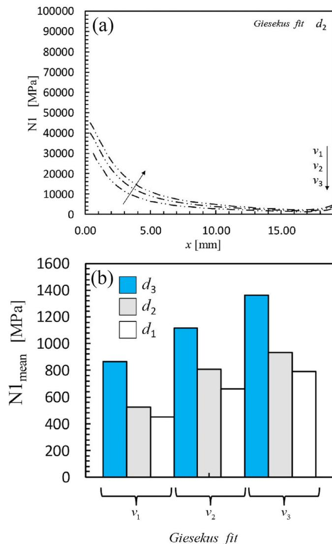
**Figure 4.** (a) Variation (along the x-axis) in the simulated normal stress difference (N1), i.e., between the rear of the spider leg and the die exit. Calculation results given here are for a fixed spider-leg location ( $d_2$ ) and for three different flow rates. (b) Calculated mean N1 ( $N1_{mean}$ ), between the rear of the spider leg and the die outlet, for the three different Giesekus models used in this work (i.e., to model the three merging location and three extrusion flow rates).
