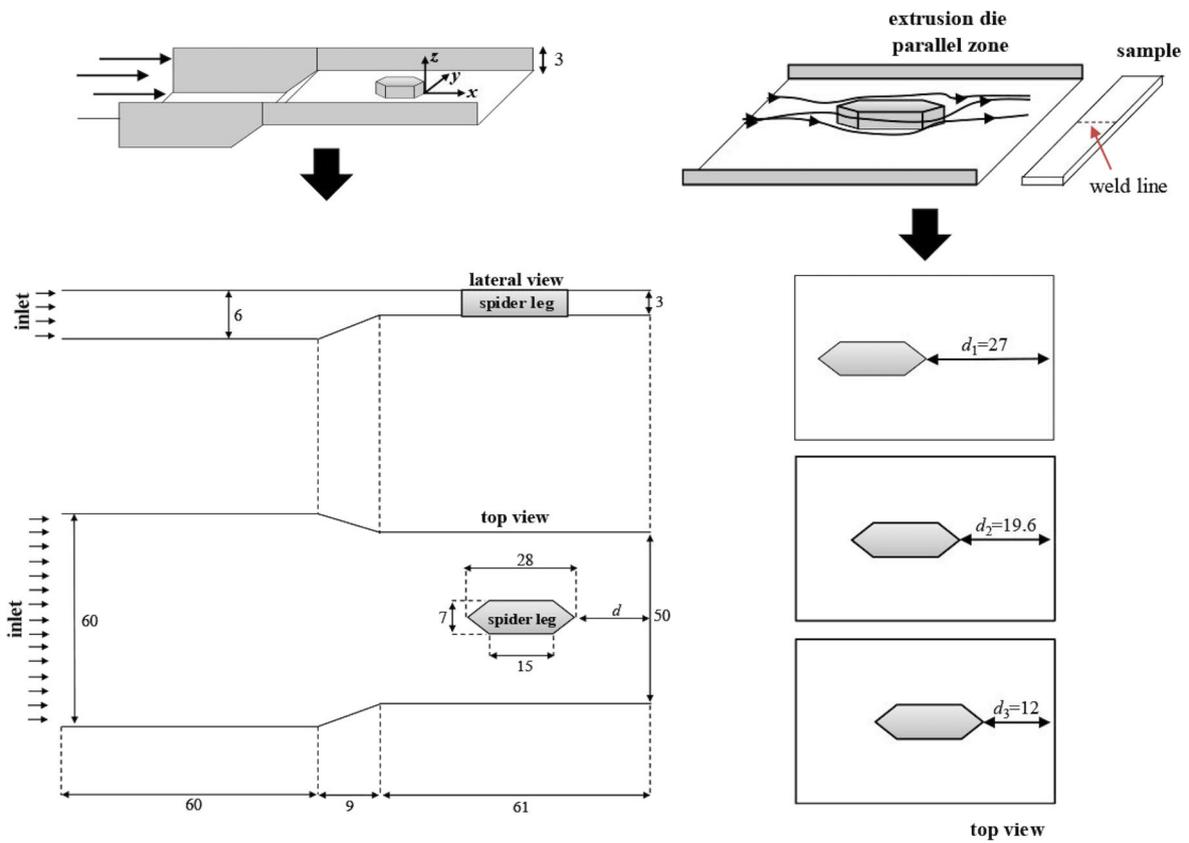
**Figure 2.** Lateral and top view of the extrusion geometry modeled in the numerical simulations. All dimensions are given in mm.  $d_1$ ,  $d_2$ , and  $d_3$ : Spider leg locations used for extrusion.
