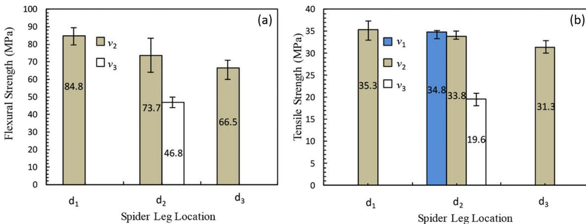
**Figure 3.** Experimental results from (a) flexural and (b) tensile strength tests. The results are given for the polystyrene samples that were extruded with the spider leg at three different positions (i.e.,  $d_1$ ,  $d_2$ , and  $d_3$ ) and for three different flow rates: 0.42 ( $v_1$ ), 0.56 ( $v_2$ ), and 0.67 ( $v_3$ ).
