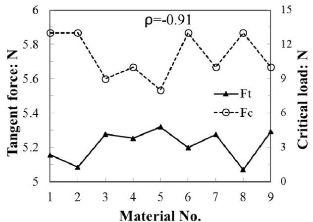
Figure 2. Comparison of the critical normal load ( $F_c$ ) and tangential force ( $F_t$ ) of the nine polypropylene (PP) samples (as listed in Table 1).  $\rho$ : Spearman correlation coefficient.
