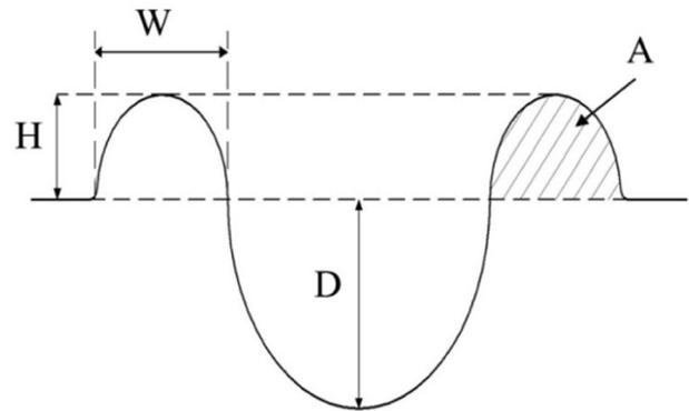
Figure 1. Schematic cross section of a scratch-induced groove.  $D$ : Residual scratch depth.  $H$ : Groove shoulder height.  $W$ : Groove shoulder width.  $A$ : Groove shoulder area.
