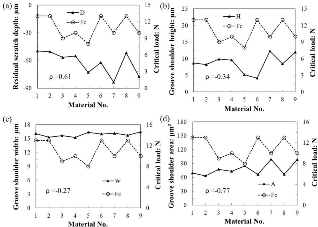
**Figure 3.** Comparisons of  $F_c$  and geometrical deformation parameters (as shown in Figure 1) for the nine PP samples. Comparisons with  $F_c$  are shown for (a) the residual scratch depth, (b) groove shoulder height, (c) groove shoulder width, (d) groove shoulder area.
