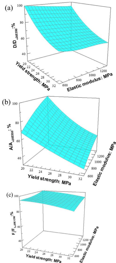
**Figure 4.** Coupling effect of  $E$  and  $\sigma_y$  on the scratch behavior of PP. Results are shown for (a)  $D$ , (b)  $A$ , and (c)  $F_t$ . All data are non-dimensionalized by their corresponding maximum values. For example,  $D/D_{\sigma_{20}E_{550}}$  means that  $D$  is normalized to the case where  $\sigma_y$  is 20MPa and  $E$  is 550MPa.
