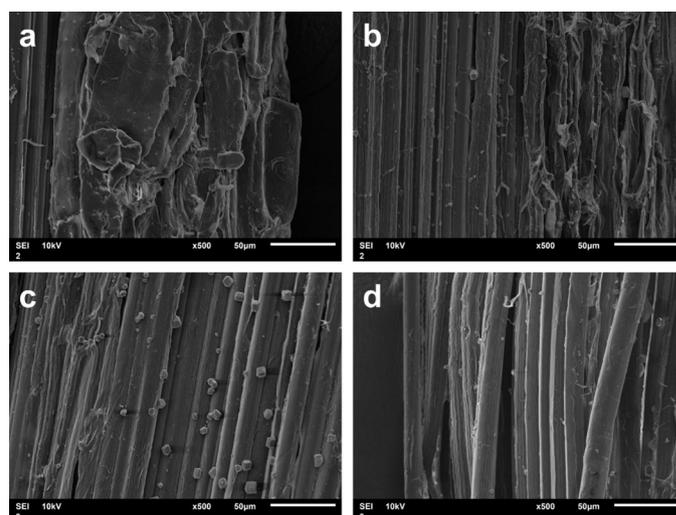
**Figure 1.** Scanning electron microscopy images of the surface morphologies of bamboo fibers treated with sodium hydroxide (NaOH). (a) Untreated, (b) 1% by weight (wt%), (c) 4wt%, and (d) 7wt% NaOH solution.
