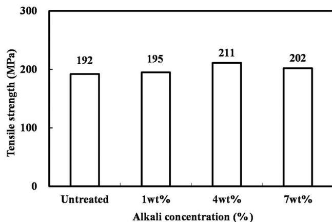
**Figure 3.** Tensile strength measurements of NaOH-treated bamboo fibers.
