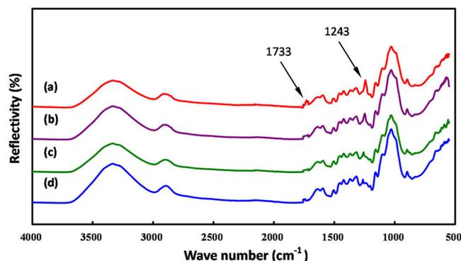
**Figure 2.** IR spectra of NaOH-treated bamboo fibers. (a) Untreated, (b) 1wt%, (c) 4wt%, and (d) 7wt% NaOH solution.
