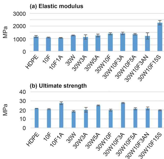
**Figure 1.** The measured (a) elastic modulus and (b) ultimate strength of the 11 composite samples (listed in Table 1).
