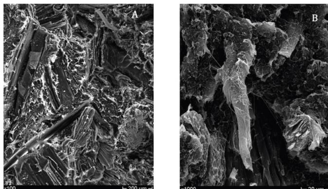
**Figure 3.** Scanning electron microscope images showing (A) the weak interfaces between both wood particles and recycled paper fibers and the HDPE matrix, and (B) the improved fiber–matrix interfaces in the 30W10F3A sample (i.e., upon addition of MAPE).
