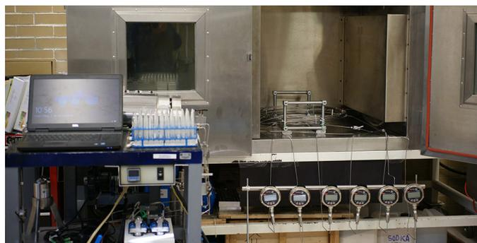
**Figure 3.** The high-pressure continuous tubular reactor used for the synthesis of polyacrylamide-based polymers.
