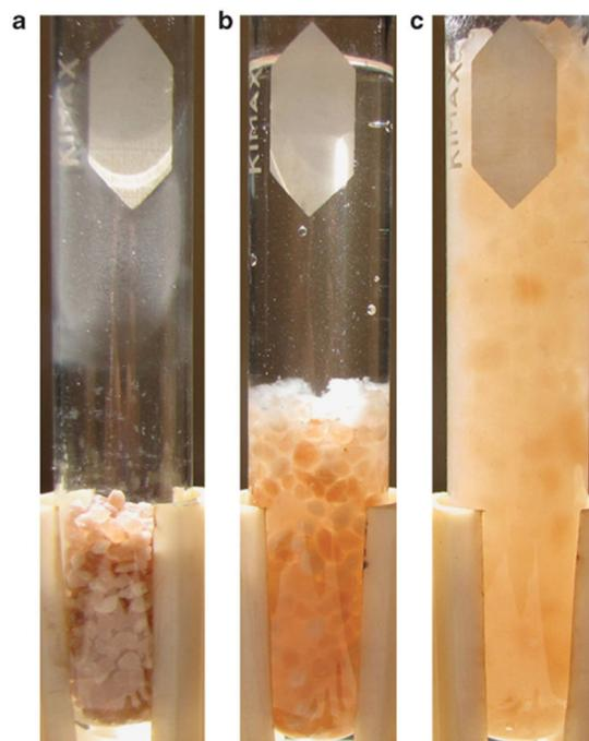
**Figure 1.** Photographs showing the swelling behavior of a gel in production water (i.e., reservoir brine). The gel comprises acrylamide/vinylpyrrolidone/sodium 2-acrylamido-2-methylpropane sulfonate, crosslinked with *N,N'*-methylenebisacrylamide. (a) Dry gel. (b) Gel at the beginning of the swelling process. (c) Gel at the end of the swelling process (i.e., after 24 hours).<sup>1</sup>
