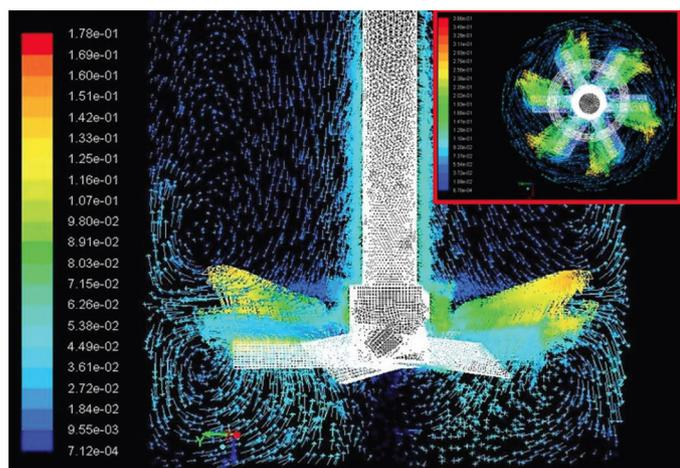
**Figure 2.** Flow patterns, simulated by computational fluid dynamics, of a stirred batch reactor.<sup>4</sup> Values shown are velocity (in  $\text{ms}^{-1}$ ).
