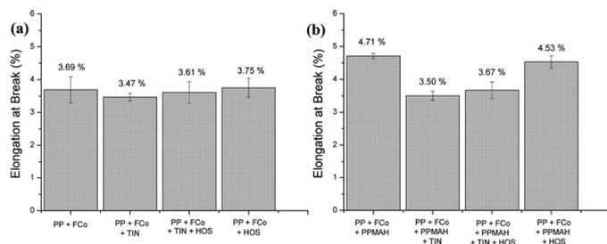
**Figure 2.** Elongation at break (%) of the (a) uncompatibilized and (b) compatibilized composite samples.
