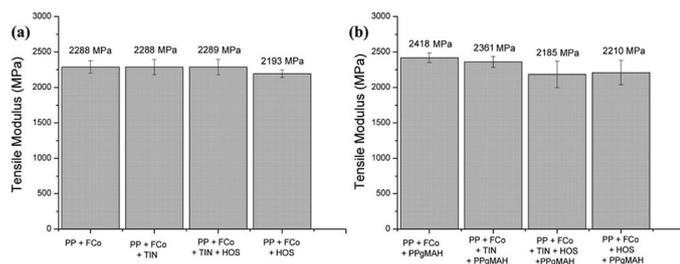
**Figure 3.** Tensile modulus of the (a) uncompatibilized and (b) compatibilized samples.
