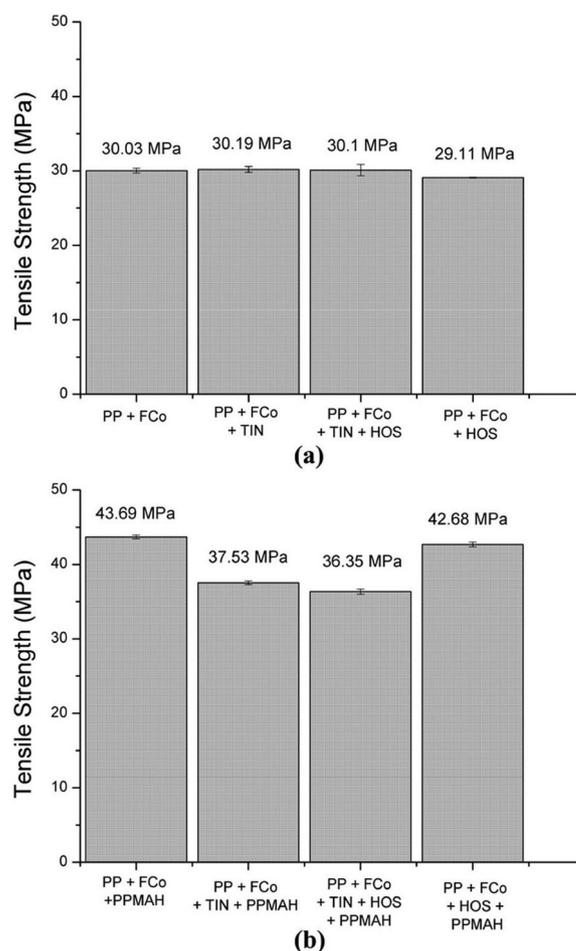
**Figure 1.** Tensile strength (MPa) of our coir/polypropylene samples with various additives. (a) Uncompatibilized samples of polypropylene/coir-fiber (PP/FCo) composites, and those fabricated with a hindered amine light stabilizer (Tinuvin® 791, TIN), and a UV absorber (Hostavin® Aro 8, HOS). (b) Composites compatibilized with maleic anhydride-grafted polypropylene (PPMAH).
