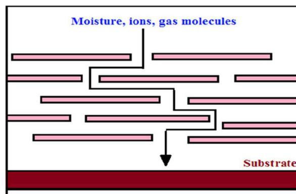
**Figure 1.** Schematic showing a polymeric/nanoclay coating on a metal substrate. A tortuous path for moisture, ions, and gas molecules is created by integrating exfoliated nanoclay platelets (pink) in an alkyd resin, thus reducing corrosion of the substrate.
