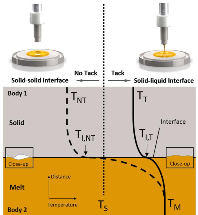
**Figure 1.** Temperature curves of the contact temperature tack (stickiness) hypothesis. No tack (NT) case: Solid temperature,  $T_{NT}$ , and melt temperature,  $T_M$  (dashed curve), and interfacial temperature,  $T_{I,NT}$ . Tack (T) case: Solid temperature,  $T_T$ , and melt temperature,  $T_M$  (solid line), and interfacial temperature,  $T_{I,T}$ .  $T_S$  denotes the solidification temperature of the melt (dotted line).
