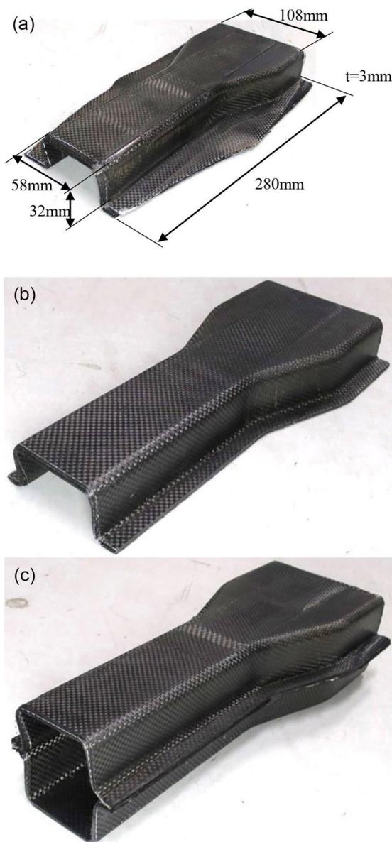
**Figure 2.** (a) A variant cross-section beam after (a) press forming and (b) trimming (by shear cutting). (c) A closed cross-section beam joined by welding.  $t$ : Thickness.
