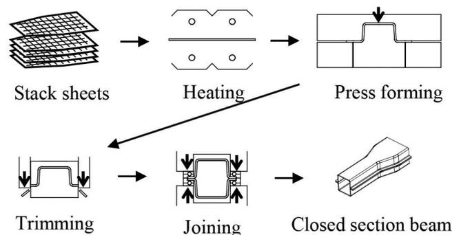
**Figure 1.** The press-forming process that we have developed and demonstrated for the formation of a variant cross-section beam.
