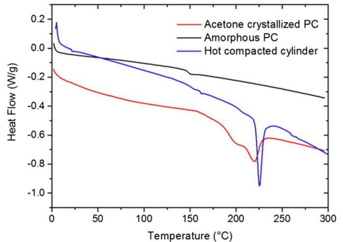
**Figure 3.** Differential scanning calorimeter analysis results for amorphous PC powder, PC powder crystallized from an acetone solution, and the HPC-produced (at 210°C) PC cylinder.
