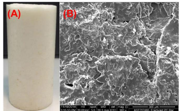
**Figure 4.** (A) Cylinder of acetone-crystallized PC powder that was produced via HPC at 180°C and discharged without cooling. (B) SEM image of the same sample, in which voids and grain boundaries (caused by under-consolidation) can be seen. Scale bar marks 300µm.
