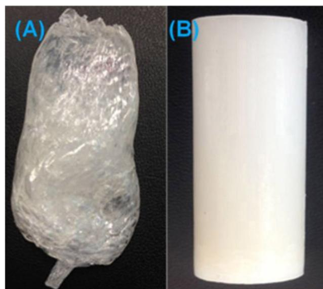
**Figure 1.** (A) Amorphous polycarbonate (PC) extruded as an irregular blob. This sample was produced by hot powder compaction (HPC), i.e., above the glass transition temperature, in a rheometer and then discharged without cooling. (B) Crystalline PC powder that was optimally compacted at 210°C into a cylinder and discharged without cooling.
