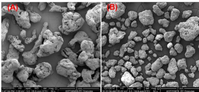
**Figure 2.** Scanning electron microscope (SEM) images of (A) amorphous PC powder and (B) PC powder crystallized from an acetone solution. Scale bars mark 2mm.
