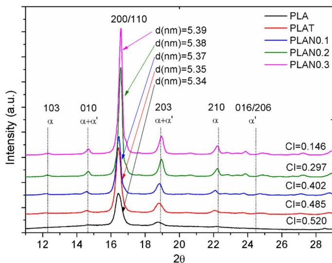
**Figure 2.** Diffraction patterns of PLA, PLAT, and nanocomposite samples. *d*: The spacing between adjacent lattice planes. *a.u.*: Arbitrary units.  $2\theta$ : Diffraction angle.  $\alpha$ : Ordered crystals.  $\alpha'$ : Disordered crystals. *CI*: Crystallinity index. Numbered peaks represent Miller indices.
