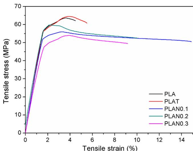
**Figure 3.** Representative stress-strain curves.
