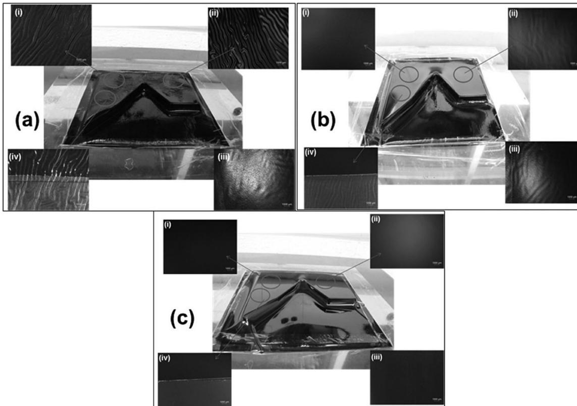
**Figure 3.** Images of FBO/PP laminate samples that were thermoformed using (a) conventional vacuum forming, (b) the isothermal bulge method, and (c) the dynamic bulge method. Insets show the (i) top sample surface, (ii) top surface at 35° inclination, (iii) back side of the laminate, and (iv) visible portion of the PP substrate where the film has been partly peeled away.
