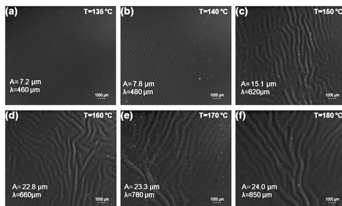
**Figure 1.** Optical images of the wrinkled blackout film/polypropylene (FBO/PP) laminates that were heated, at a rate of 70°C/minute, to a temperature (T) of (a) 135°C, (b) 140°C, (c) 150°C, (d) 160°C, (e) 170°C, and (f) 180°C. A and λ: Amplitude and wavelength of wrinkles, respectively. Scale bars indicate 1000 μm.
