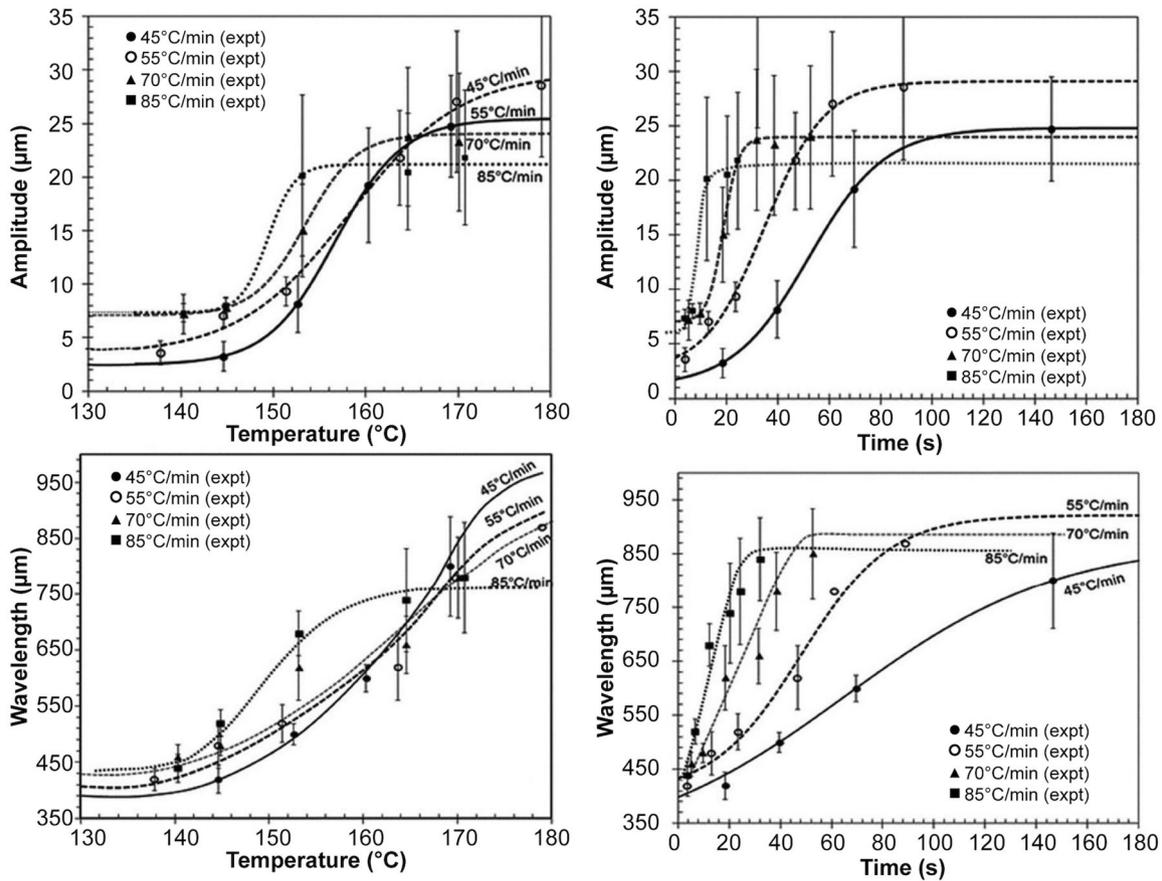
**Figure 2.** Variation in the amplitude (top) and wavelength (bottom) of the wrinkles on four FBO/PP samples (those heated at rates of 45, 55, 70, and 85°C/min) as a function of temperature (left) and time (right). Expt: Experimental.
