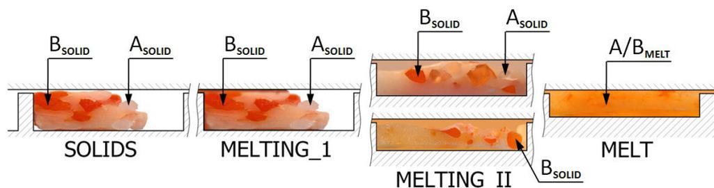
**Figure 2.** Schematic depiction of the four-section melting mechanism for polymer blends in a starve-fed single-screw extruder. A and B: Major and minor components of the polyblend material. SOLIDS: Solid conveying of the material occurs in the partially filled region. MELTING\_I: Melting occurs via conduction. MELTING\_II: Both conduction and dispersive melting of one/two of the blend components occurs. MELT: Melt flow takes place.<sup>8</sup>
