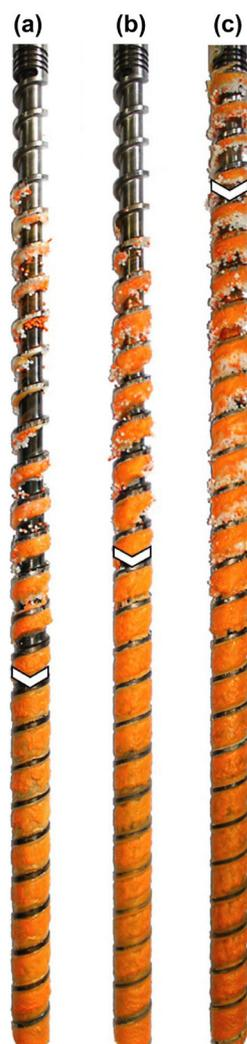
**Figure 1.** Photographs of the screws pulled out of the machine after extrusion of the polypropylene/polystyrene blend, at a screw speed of 50rpm and metered feed rates of (a) 11kg/h, (b) 12kg/h, and (c) a flood-fed rate of 13kg/h. Arrows mark the beginning of the fully filled region.<sup>8</sup>
