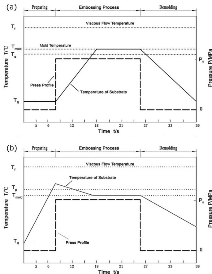
**Figure 2.** The new plate to plate transition-spanning isothermal hot embossing (P2P TSI HE) process for amorphous polymers. (a) The substrate is not preheated and the mold temperature ( $T_{\text{mold}}$ ) is higher than  $T_g$ . (b) The substrate is preheated and  $T_{\text{mold}}$  is lower than  $T_g$ .
