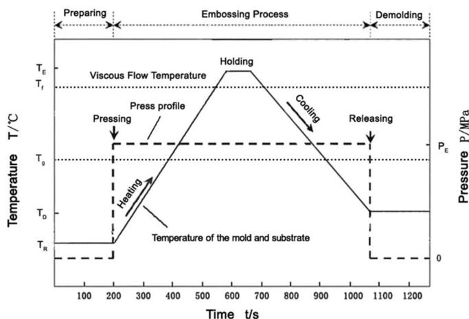
**Figure 1.** The conventional plate to plate hot embossing process.  $T_R$ : Room temperature.  $T_D$ : Demolding temperature.  $T_g$ : Glass transition temperature.  $T_f$ : Viscous flow temperature.  $T_E$ : Embossing temperature.  $P_E$ : Embossing pressure.
