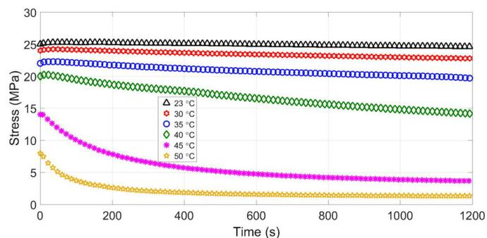
**Figure 3.** Experimental data (stress versus relaxation time) from the PLA loading/partial unloading–relaxation tests (at 23–50°C).
