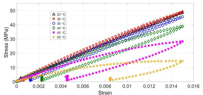
**Figure 1.** Experimental results from loading–unloading tests of poly(lactic acid), PLA, at various temperatures (i.e., 23–50°C). For these tests, the sample was stretched with a maximum strain ( $\epsilon_{max}$ ) of 0.015 and unloaded with a minimum stress ( $\sigma_{min}$ ) of 1MPa.
