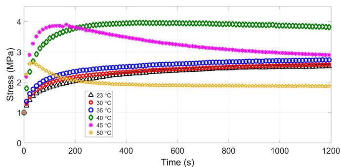
**Figure 2.** Results (stress as a function of relaxation time) from the relaxation under retraction tests for PLA, at a range (23–50°C) of temperatures.
