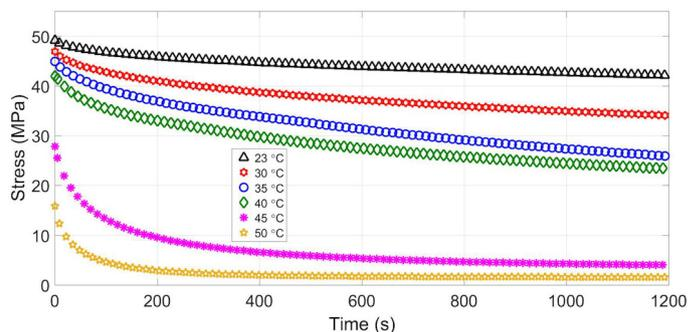
**Figure 4.** Stress–relaxation time data obtained during the PLA relaxation (under tension) tests at 23–50°C.
