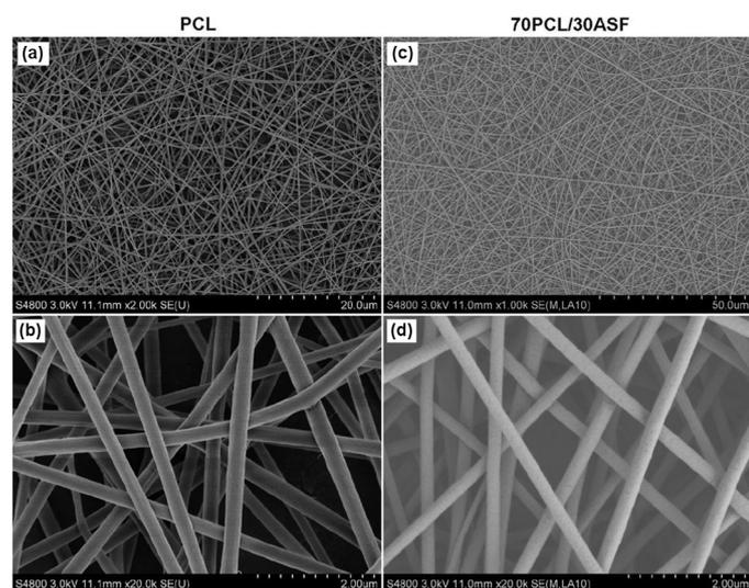
**Figure 2.** Scanning electron microscopy images of (a, b) electrospun 100% PCL and (c, d) 70% PCL/30% ASF (70PCL/30ASF) nanofibers.
