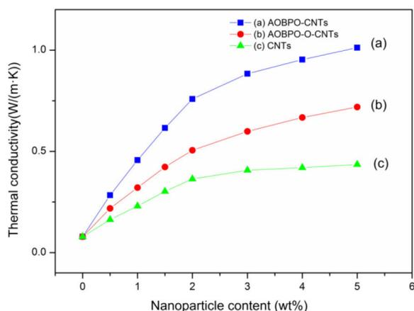
**Figure 4.** Thermal conductivities of silicone resin nanocomposites filled with CNTs, AOBPO-CNTs, and AOBPO-O-CNTs of different mass fractions (from 0 to 5wt%) at 25°C.
