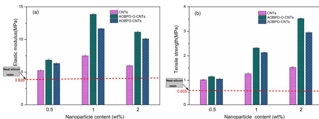
**Figure 3.** (a) Elastic modulus and (b) tensile strength of neat silicone resin and nanocomposites of silicone resin and CNTs, AOBPO-O-CNTs, and AOBPO-CNTs.
