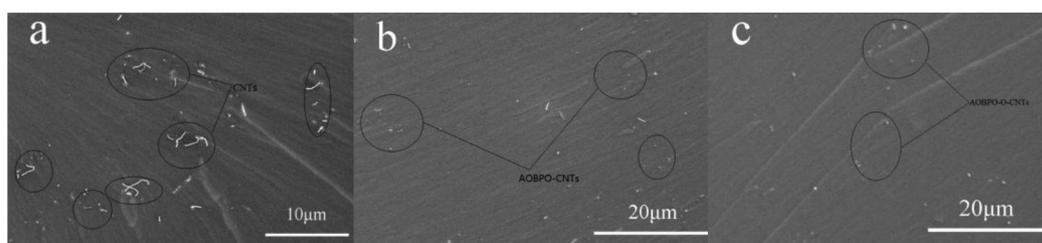
**Figure 2.** Scanning electron micrographs of (a) pristine CNTs, (b) AOBPO-CNTs, and (c) AOBPO-O-CNTs dispersed in silicone resin.
