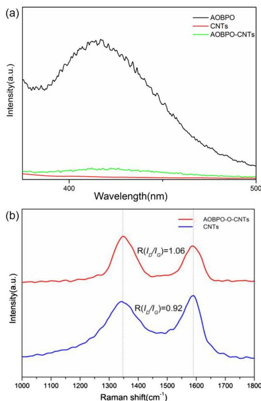
**Figure 1.** (a) Room-temperature photoluminescent emission spectra, obtained using an excitation wavelength of 325nm, and (b) Raman spectra of carbon nanotubes (CNTs). AOBPO-CNTs and AOBPO-O-CNTs: CNTs that have undergone functionalization with a liquid crystal molecule (4'-allyloxy-biphenyl-4-ol, AOBPO) via physical and chemical means, respectively.  $R(I_D/I_G)$ : Band-intensity ratio of the two first-order bands.
