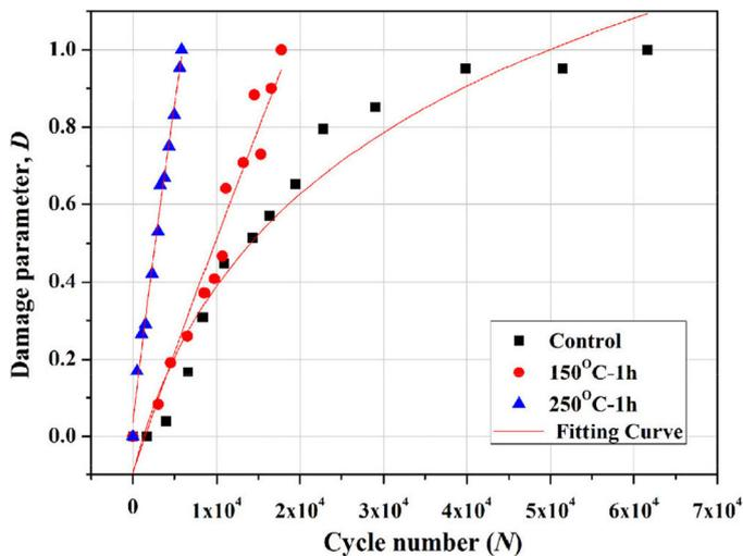
**Figure 2.** Evolution of the damage in the BFRP as a function of the number of fatigue cycles for three BFRP samples (at a strain ratio of 66.4%). Both the experimental results and fitting curves are shown.
