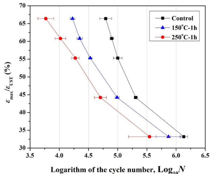
**Figure 1.** The change in the fatigue lifetime (expressed in terms of  $N$ , the number of fatigue cycles before failure) of a control sample and basalt-fiber-reinforced polymer (BFRP) plates that were subjected to elevated temperatures (150 and 250°C) for 1 hour, under different strain ( $\epsilon$ ) ratios.  $\epsilon_{\max}$ : Maximum strain.  $\epsilon_{UST}$ : Ultimate static tensile strain.
