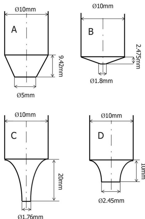
**Figure 1.** Diagrams of the flow channel within the different nozzle geometries used in the elongational deformation experiments. The geometry of the (A) standard injection nozzle, (B) short, conically shaped nozzle, (C) long, hyperbolically shaped nozzle, and (D) short, hyperbolically shaped nozzle are shown.<sup>9</sup>  $\phi$ : Diameter.
