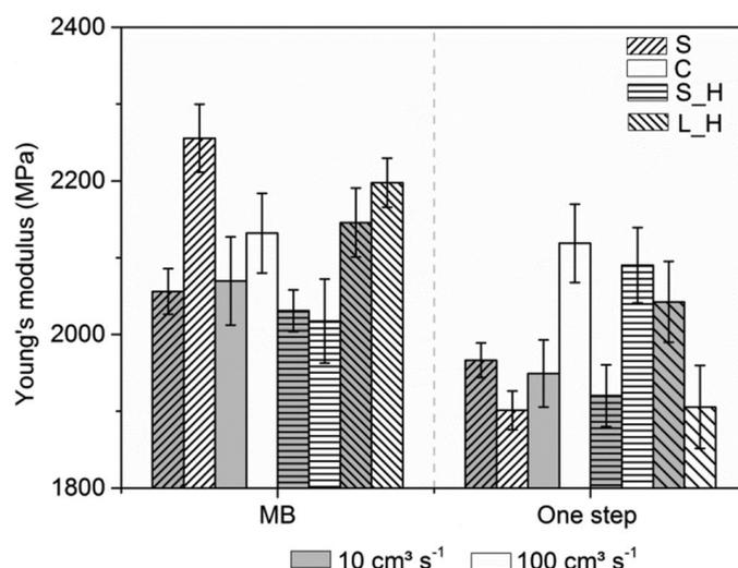
**Figure 2.** Young's modulus of the polymer nanoclay composites (PNCs) produced with the use of the standard (S), conical (C), short, hyperbolically shaped (S\_H), and long, hyperbolically shaped (L\_H) nozzles at volumetric flow rates of 10 or 100cm<sup>3</sup>s<sup>-1</sup> in the (left) MB and (right) one-step injection molding processes.<sup>9</sup>
