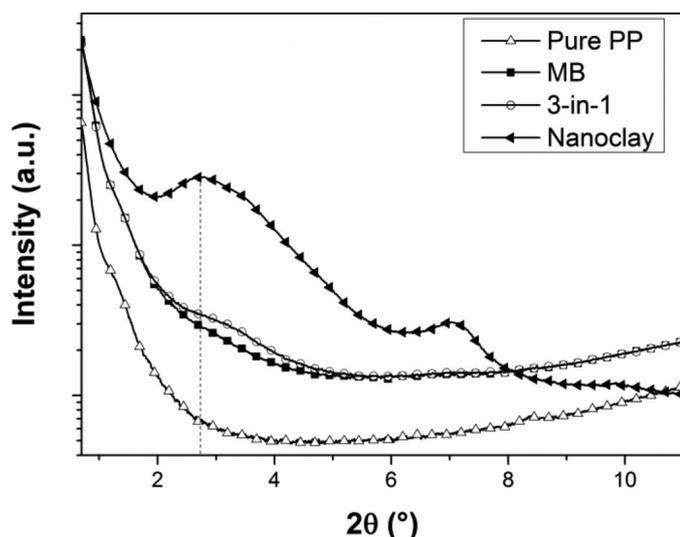
**Figure 3.** Small-angle x-ray scattering measurements of pure polypropylene (PP), nanoclay, and PNCs produced via the MB process and the one-step process (3-in-1). These results were obtained with the use of the short, hyperbolically shaped nozzle, and a volumetric flow rate of  $100\text{cm}^3\text{s}^{-1}$ .<sup>9</sup> a.u.: Arbitrary units.  $\theta$ : Scattering angle.
