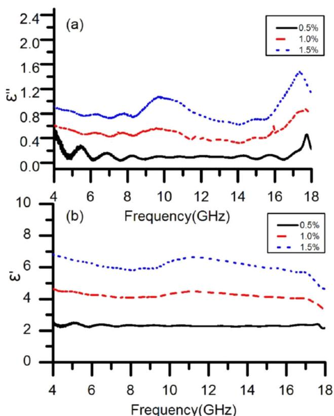
**Figure 2.** The (a) imaginary ( $\epsilon''$ ) and (b) real ( $\epsilon'$ ) parts of the permittivity of the CNT/photopolymer composites (with 0.5, 1.0, and 1.5wt% CNTs), shown as a function of frequency.
