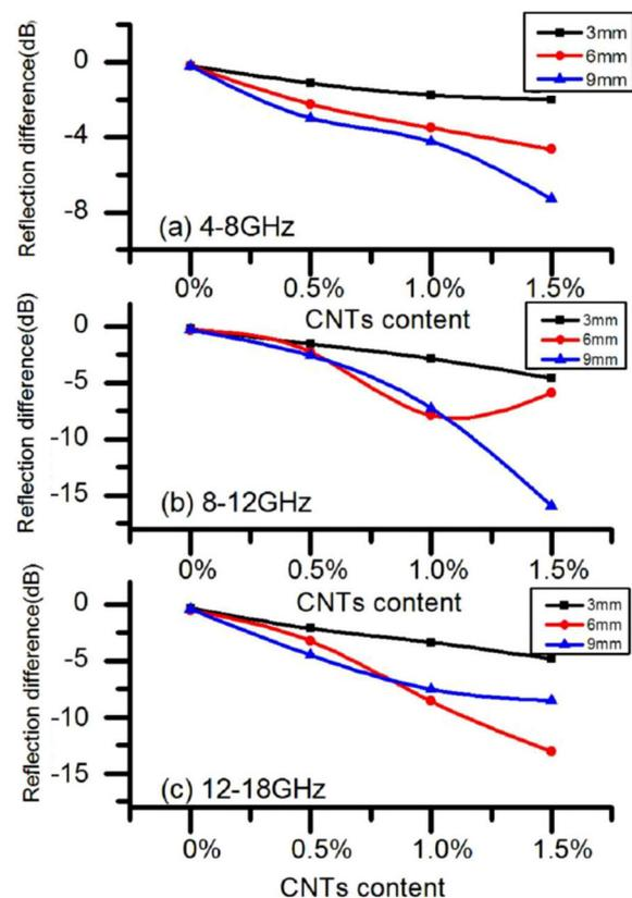
**Figure 1.** Free-space time-domain reflectivity measurements from the carbon nanotube (CNT)/photopolymer composites. The reflection difference results are shown as a function of CNT content for samples with different thicknesses (i.e., 3, 6, and 9mm) at frequencies of (a) 4–8GHz, (b) 8–12GHz, and (c) 12–18GHz.
