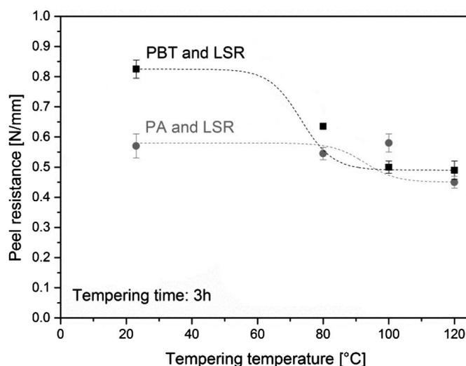
**Figure 1.** Influence of tempering at a range of temperatures (80, 100, and 120°C) on the peel resistance of liquid silicone rubber (LSR) from poly(butylene terephthalate)—PBT—and polyamide (PA). The tempering time was three hours (3h). Reference combinations of PA/LSR and PBT/LSR (the first two points in the graph) were not tempered and were stored at room temperature.
