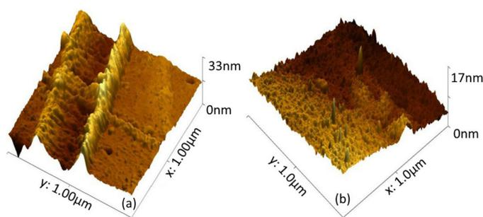
**Figure 1.** Atomic force microscope images of (a) a sulfonated poly(ether ether ketone)—SPEEK—membrane, and (b) a modified SPEEK membrane (SPEEK/BMI<sup>+</sup>). This membrane incorporates the ionic liquid 1-butyl-3-methylimidazolium tetrafluoroborate (BMI.BF<sub>4</sub>). Immersion in the ionic liquid reduced the membrane's surface roughness.
