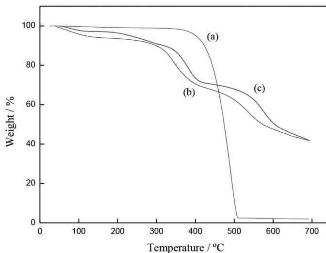
**Figure 3.** Thermogravimetric analysis curves of (a) BMI.BF<sub>4</sub>, (b) SPEEK, and (c) SPEEK/BMI<sup>+</sup> membranes. The modified membrane exhibits an improved thermal stability compared with the pristine SPEEK membrane.
