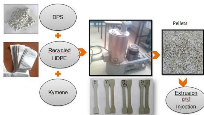
**Figure 1.** Schematic illustration of the melt compounding manufacturing process for the de-inking paper sludge/recycled high-density polyethylene (DPS/RHDPE) pellets. Different DPS loadings (0–20wt%) and compatibilizer contents (0–4wt%) are used for different formulations, and Kymene—a commercial paper wet-strength agent polyamideamine-epichlorohydrin (PAE) resin—is used as the DPS binder.
