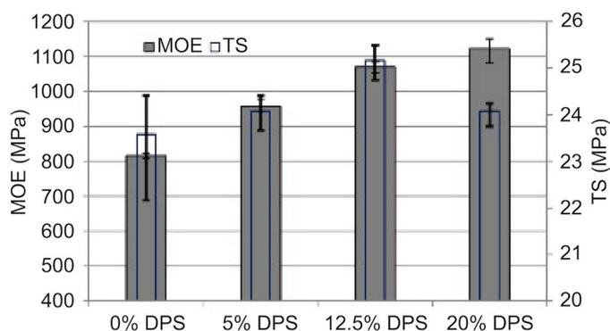
**Figure 3.** The effect of DPS, and a 2% PAE content, on the tensile strength (TS) and elastic modulus (MOE) of the DPS/RHDPE composites.
