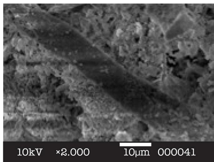
**Figure 2.** Scanning electron microscope image of DPS that shows the irregular, cracked, and short fibers mixed with mineral aggregates.
