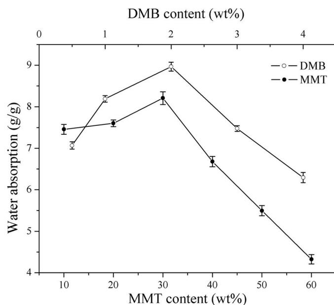
**Figure 2.** The effect of changing DMB and MMT content on the water absorption of poly(AM/O-MMT).
