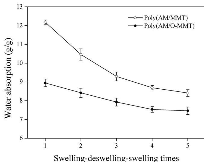
**Figure 3.** The re-swelling ability (for 1–5 cycles) of polyacrylamide-montmorillonite—poly(AM/MMT) and poly(AM/O-MMT) composites in distilled water at 95°C.
