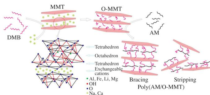
**Figure 1.** Schematic illustration of the synthesis process for polymer-montmorillonite hybrid—poly(AM/O-MMT)—materials. DMB: 2-(dimethylamino) ethyl methacrylate with 1-bromohexadecane (a long alkyl chain ammonium salt). MMT: Montmorillonite. O-MMT: Intermediate-MMT. AM: Acrylamide. Al: Aluminum. Fe: Iron. Li: Lithium. Mg: Magnesium. OH: Hydroxyl. O: Oxygen. Na: Sodium. Ca: Calcium.
