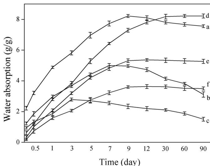
**Figure 4.** The time and salinity dependence of water absorbency for (a–c) poly(AM/MMT) and for (d–f) poly(AM/O-MMT) composites. Results are given for salinities of (a) and (d) 0 mg/L, (b) and (e)  $1 \times 10^5$  mg/L, and (c) and (f)  $2 \times 10^5$  mg/L.
