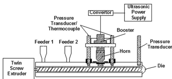
**Figure 1.** Schematic diagram of the ultrasonic twin-screw extruder.
