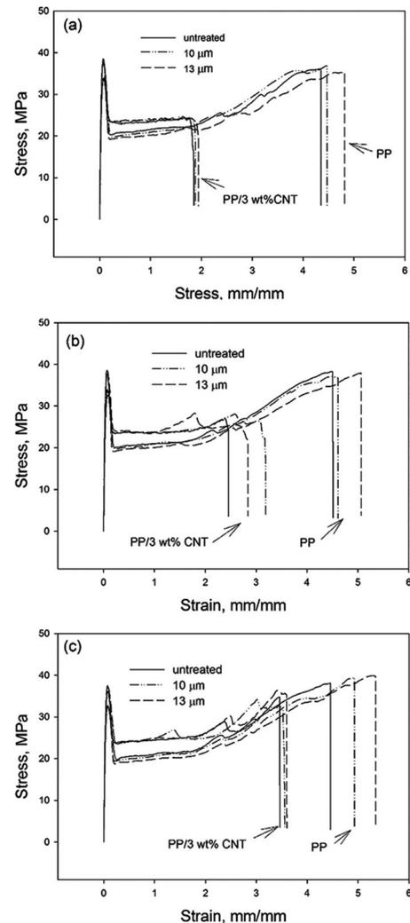
**Figure 5.** Stress-strain curves of PP and PP/3wt% composites prepared using (a) Design 1, (b) Design 2, and (c) Design 3. CNT: Carbon nanotube.
