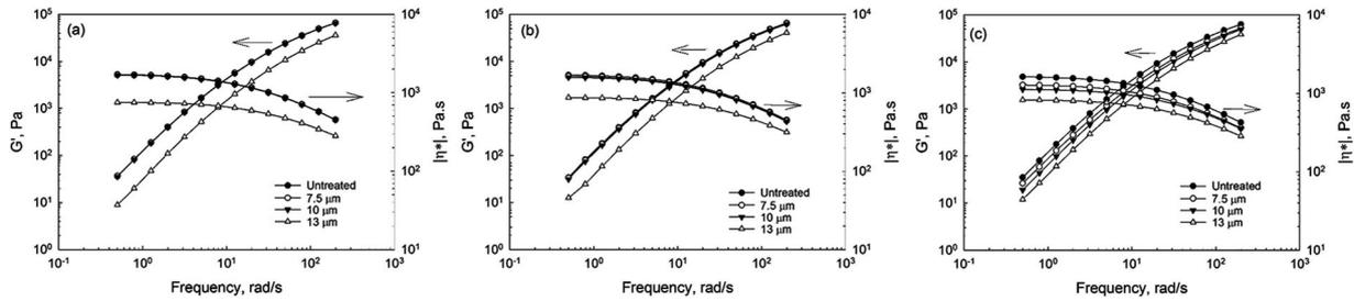
**Figure 3.** Storage modulus ( $G'$ ) and complex viscosity ( $|\eta^*|$ ) of untreated and treated (at amplitudes of 7.5, 10, and 13  $\mu\text{m}$ ) pure polypropylene (PP) in three screw designs: (a) Design 1, (b) Design 2, and (c) Design 3.
