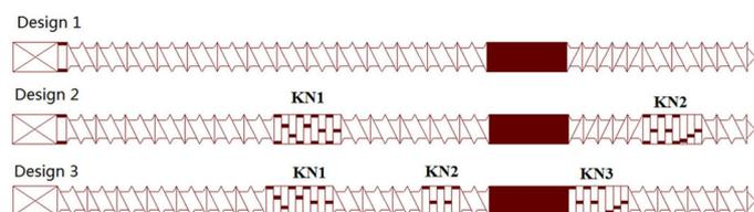
**Figure 2.** Schematic illustration showing three different screw configurations. KN1:  $5 \times 60^\circ$  RH +  $4 \times 90^\circ$  RH. KN2:  $5 \times 90^\circ$  RH. KN3:  $4 \times 90^\circ$  RH +  $4 \times 30^\circ$  LH. RH: Right-handed elements. LH: Left-handed elements.
