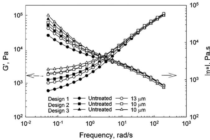
**Figure 4.**  $G'$  and  $|\eta^*|$  for untreated composites and composites prepared using Design 1 at an amplitude of 13  $\mu\text{m}$  and with Designs 2 and 3 at an amplitude of 10  $\mu\text{m}$ .
