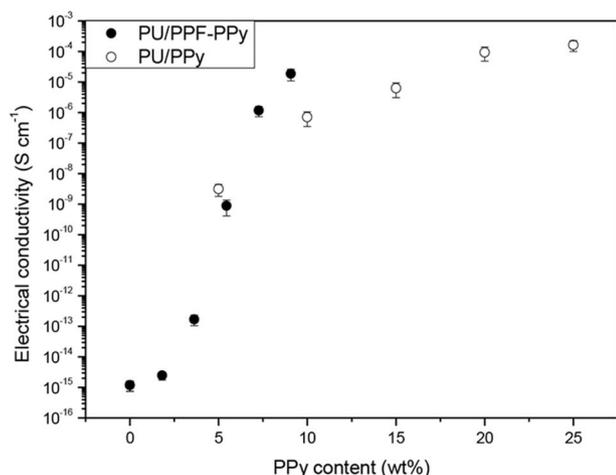
**Figure 2.** Electrical conductivity, shown as a function of PPy content, of polyurethane (PU) matrix composites that contain either PPF-PPy or neat PPy filler particles.<sup>12</sup>
