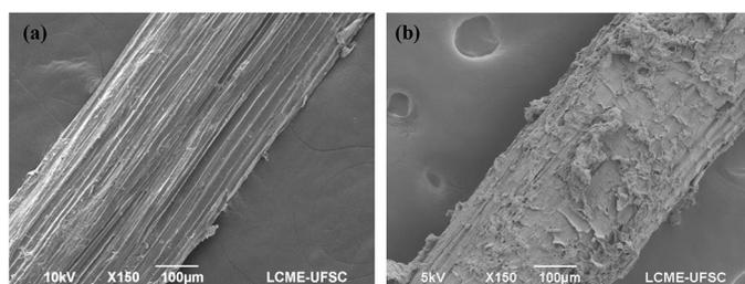
**Figure 1.** Scanning electron micrographs of peach palm fibers (PPFs) that are (a) uncoated and (b) coated with polypyrrole (PPy).<sup>12</sup>
