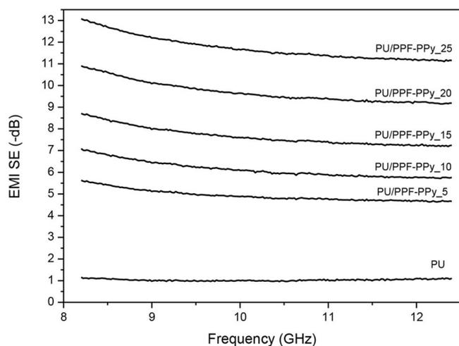
**Figure 3.** Electromagnetic interference shielding effectiveness (EMI SE) of PU/PPF-PPy composites that have 5, 10, 15, 20, and 25wt% conductive filler content.<sup>12</sup>
