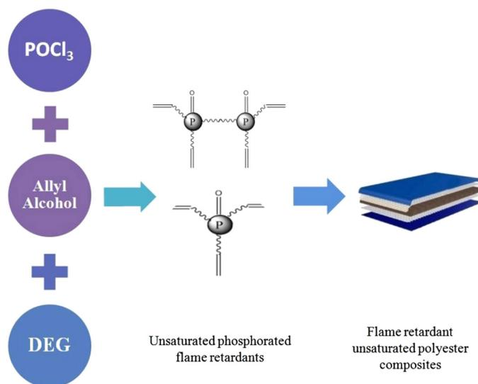
**Figure 1.** Phosphoryl chloride ( $\text{POCl}_3$ ), allyl alcohol, and diethylene glycol (DEG) were used to synthesize two novel, phosphorus-containing reactive flame retardants. These were then incorporated into unsaturated polyester to obtain composites with improved flame retardancy. P: Phosphorus.
