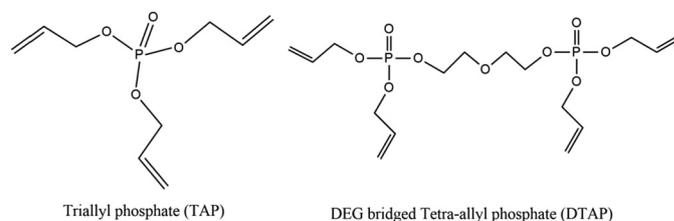
**Figure 2.** Chemical structures of the two synthesized flame retardants: triallyl phosphate (TAP) and DEG-modified tetra-allyl phosphate (DTAP).
